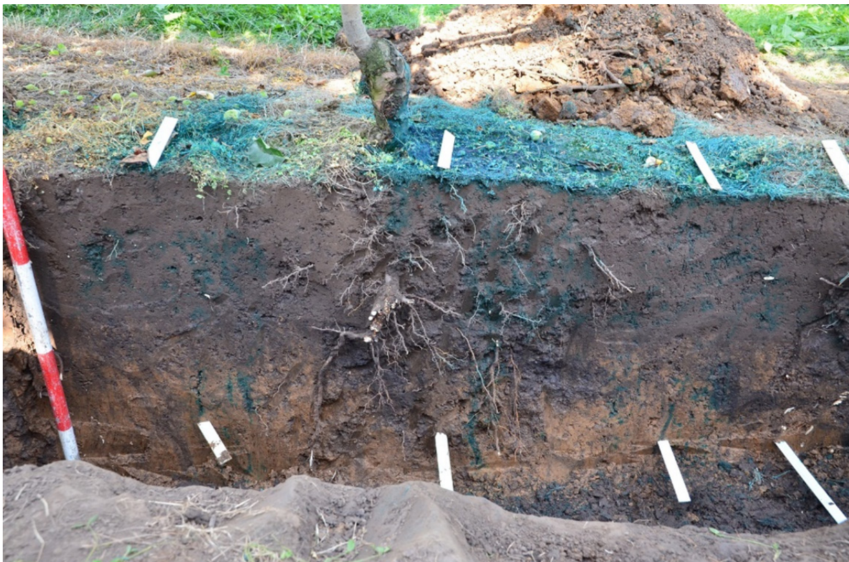
Figure 32. Soil profile and root zone wetted with water mixed with food coloring. The white labels on the soil surface indicate the location of the drippers. The bottom row of tags indicates the soil depth at 30 cm as seen with the attached tracer stick.
