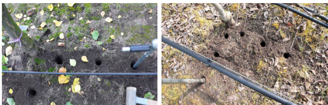
Figure 30. Soil with roots sampling using a soil drill at different distances from the tree trunk.
